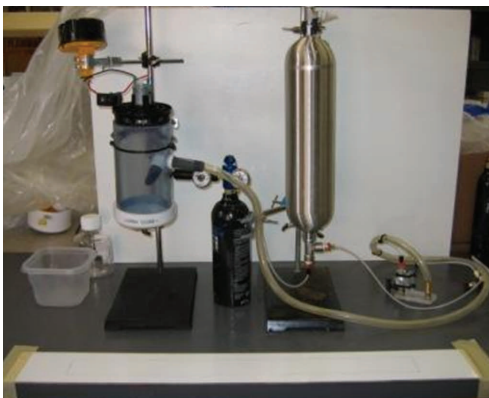
Figure 2. The prototype surface extraction system designed and built at AlburtyLab was one method used for surface sampling. One of the spiked coupons is visible in the foreground
